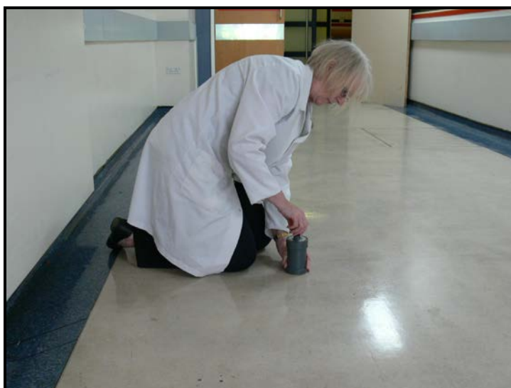
Figure 6. Sampling using the Camraso Soil Monitor
